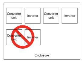
Arrangement of multiple inverters and converter units
