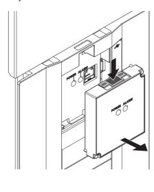
• To install the inverter operation panel (FR-DU08), align its connector on the back with the PU connector of the inverter, and insert the operation panel. After confirming that the operation panel is fit securely, tighten the screws. (Tightening torque: 0.40 to 0.45 N•m)
