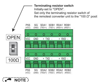
• To avoid malfunction, keep the RS-485 terminal wires away from the control circuit board.
