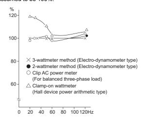
Example of measuring inverter output power
