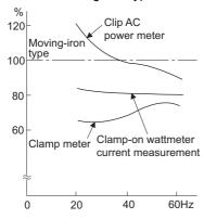
Example of measuring converter unit input current
