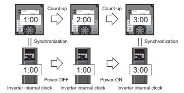
• When the time is set using the inverter parameters, the time of FR-LU08 is set to the time of inverter internal clock.
