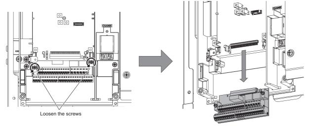
2) Be careful not to bend the pins of the converter unit's control circuit connector, reinstall the control circuit terminal block, and fix it with the mounting screws.
