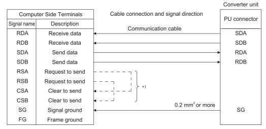
\*1 Make connection in accordance with the Instruction Manual of the computer to be used with. Fully check the terminal numbers of the computer since they vary with the model.
