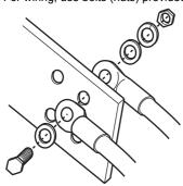
• When wiring cables to the main circuit conductor (R/L1, S/L2, T/L3) of the converter unit, use the bolts (nuts) for main circuit wiring, which are provided on the front side of the conductor.
