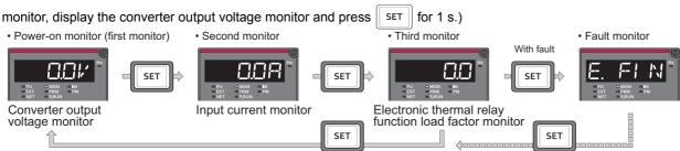
• Pr.774 sets the first monitor, Pr.775 sets the second monitor, and Pr.776 sets the third monitor to be displayed.
