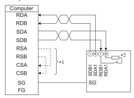
• Wiring of n converter units (multiple units) and one computer with RS-485 terminals
