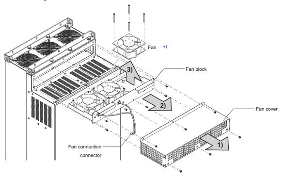
\*1 The number of cooling fans differs according to the converter unit capacity.
