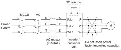
\*1 The converter unit (FR-CC2) is equipped with the DC reactor.
