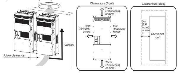
\*1 For replacing the cooling fan, 30 cm (11.81 inches) or more of space is necessary in front of the converter unit. Refer to page 157 for fan replacement.
