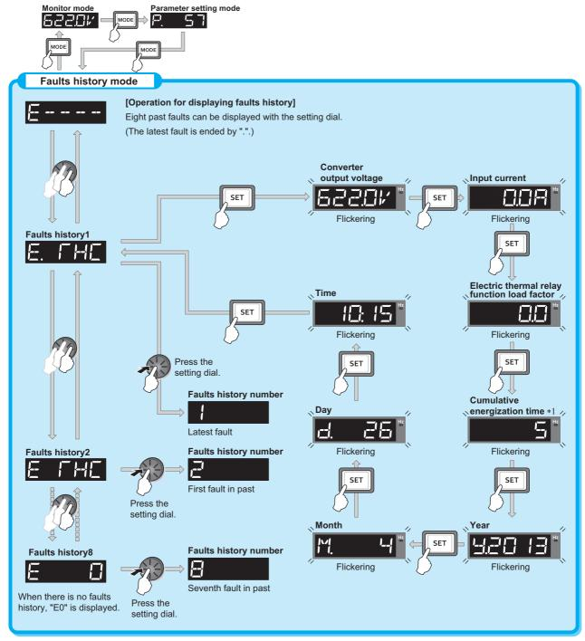
The cumulative energization time is accumulated from 0 to 65535 hours, then cleared, and accumulated again from 0.
